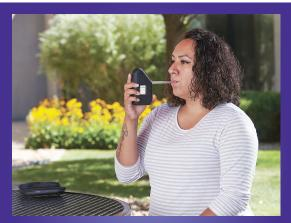
The alcohol monitor is a handheld portable device that fits in a pocket or purse. The participant blows into the device, it detects the alcohol level and takes a photo.
